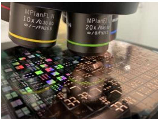
The first processed device wafers of fully vertical GaN-on-silicon MOSFETs
